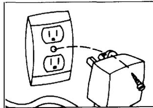
Then, plug the power transformer into a regular wall outlet. It is best to plug the transformer into a wall outlet that is continuously "live," not one controlled by a wall switch. You may want to secure the power transformer to the wall outlet as in the sketch above. (*Note:* Some wall plates may not have a screw location that matches the transformer.)
