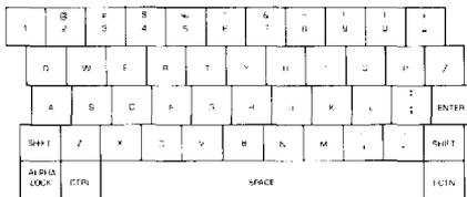
The keyboard is like a standard typewriter, with keys of several types. Pressing any key causes its *lower-case* (small capital) character to display on the screen, and holding down the **SHIFT** key while pressing any other key returns the *upper-case* (large capital) character for that key. Except for the alphabetical keys, each key's upper-case character is printed at the top of the key face, while the lower-case character is printed at the bottom.
