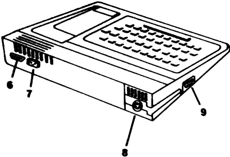
6 The Cassette Interface Cable\* connects to the console at this 9-pin "D" outlet. (See pages 14-16 for more details.)
